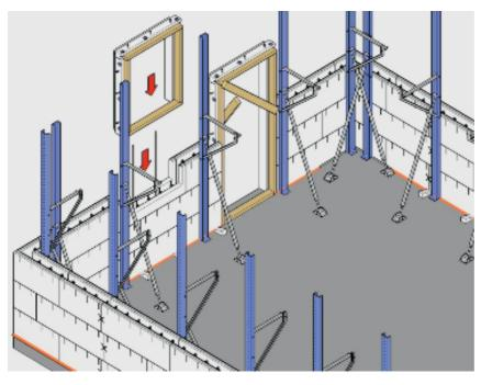
Now place the props as shown. Average spacing should be 1.4m but beside door props openings are essential and window opening may also require them. Props must be attached to Use each course. screws for hexagonal ease of application - and they are easily removed stored and used multiple times. Props need to be close to corners (no more than 400mm away
