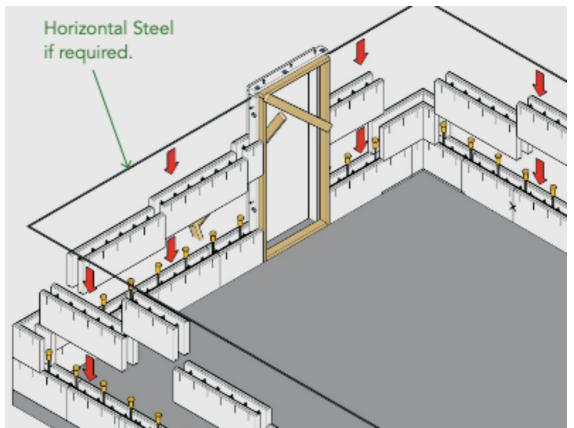
Repeat for course 3 and 4 adding rebar as specified although no further adjustment should be needed for horizonal leveling. Course 1,3,5 etc. should be the same and course 2,4 and 6 will be the same as each other but with staggered joints from 1, 3, 5 etc. Window formwork may be needed at this point. Add to starter bars under windows to bring up to sill height and add sill bar as specified before placing window formwork.
