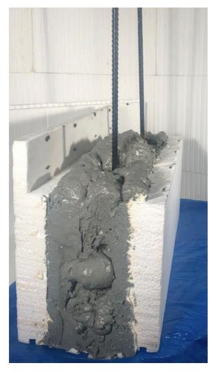
To achieve both the desired R rating and the cover necessary to bolt a 90mm frame to the slab a 100mm deep rebate is cut on the inside edge of the top of the out block. This is only necessary for 90mm timber walls and 140mm timber can be fastened to the slab without and changes needed.
