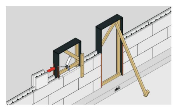
Accurately cutting the blocks against the formwork means that foaming between blocks and formwork will not be necessary. The props holding the walls vertical are adjustable during concrete pouring and should be on either side of door openings so blocks and formwork don't need to be glued together.
