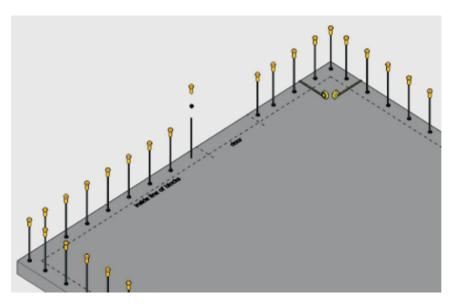
A typical layout would look like this. A good idea at this point is to slip a 30mm length of plastic pipe over the starters that is has an internal diameter at least 2 times the diameter of the rebar. This will allow the easy insertion of verticals when several courses have been added.
