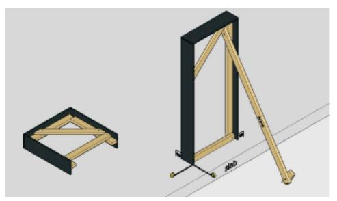
You may find on a windy day that the formwork needs to be held in place while the blockwork is built around it as below.
