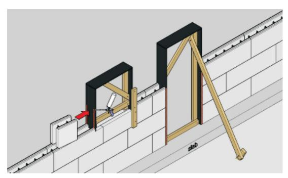
Accurately cutting the blocks against the formwork means that foaming between blocks and formwork will not be necessary. The props holding the walls vertical are adjustable during concrete pouring and should be on either side of door openings so blocks and formwork don't need to be glued together.
