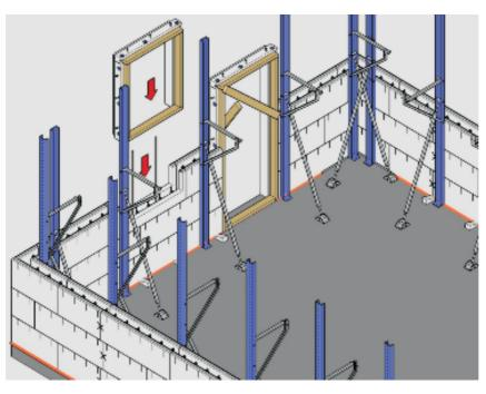
Now place the props as shown. Average spacing should be 1.4m but props beside door openings are essential and window opening may also require them. Props must be attached to each course. Use hexagonal screws for ease of application – and they are easily removed stored and used multiple times. Props need to be close to corners (no more than 400mm away
