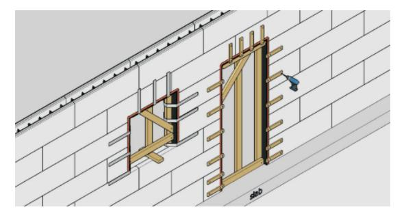
Now lay the first course. Starting with the corner blocks, lay the first row. Cut blocks to align the cut ends with openings and wall ends where possible. Otherwise make a staggered joint in the middle of a wall.
