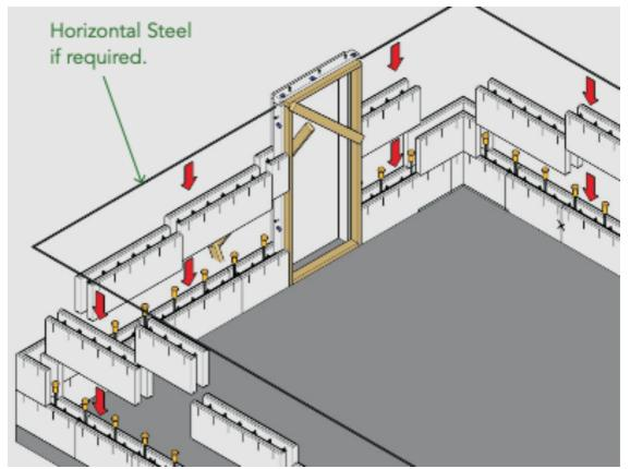
Window formwork may be needed at this point. Add to starter bars under windows to bring up to sill height and add sill bar as specified before placing window formwork.
